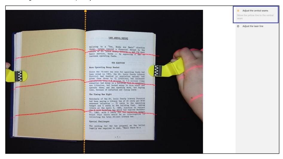
23. If the curve correction of an image is skewed, you can adjust the laser lines. Click **Adjust the laser line** on the right.
