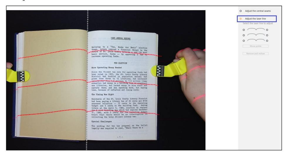
Then, below that button, click on the line you want to adjust. When you've selected the line, you can either move the orange points on the line, or remove and replace the dots completely.
